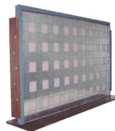
4x8x2 PURA Dual polarized uniform rectangular patch array
