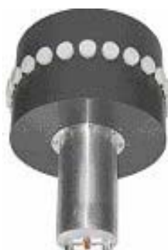
24x2 PUCPA Dual polarized uniform circular patch array
