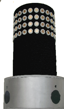
4x24x2 SPUCPA Stacked Polarimetric Uniform Circular Patch Array
