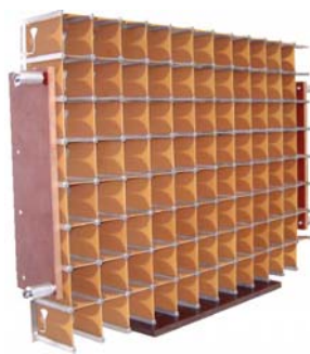
4x8x2 PURA Dual polarized uniform rectangular Vivaldi array
