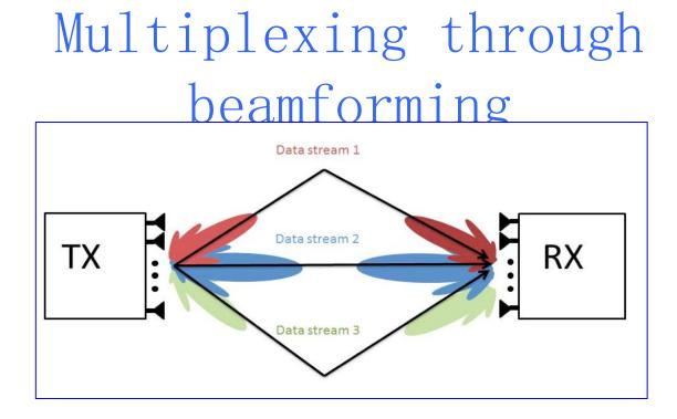
Here **beamforming** is enforced to multiplex different data-streams over different paths
