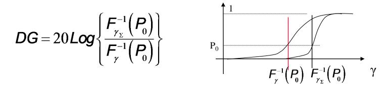
The DG depends on the combining technique and on the residual fading correlation between the different branches. If the branches are correlated then  $F_{\gamma}(\gamma)$  and  $F_{\gamma_{\Sigma}}(\gamma)$  are the same and there is no gain
