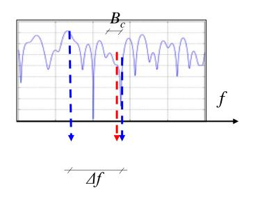
• We have <u>intrinsic frequency diversity when  $B > B_c$ </u>. This also means selective fading, but in digital systems this can even improve BER.
