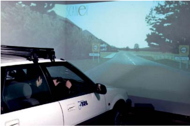
Use of a driving simulator to assess distraction from use of a mobile phone while driving (photograph courtesy of Mr Andrew Parkes, TRL Ltd)
