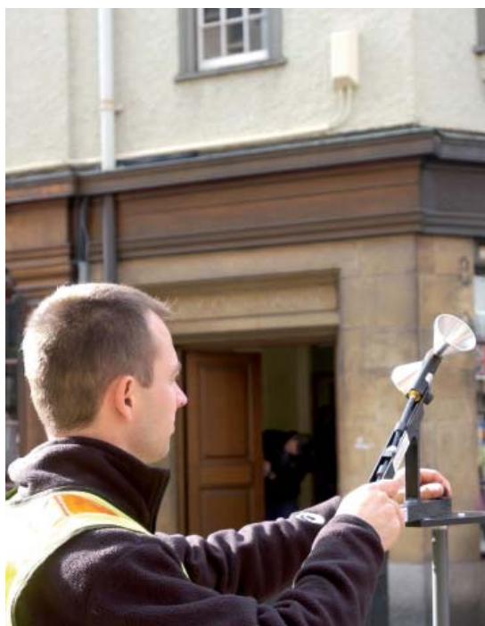
Measurement of fields emitted from microcell base station (photograph courtesy of the Health Protection Agency)
